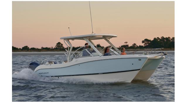
LOA: 26' 0" Beam: 8' 6" Fuel Capacity: 186 gal (2 x 93 gal) Dry Weight w/ Power (Approx.): 6,600 lbs w/ twin 150's Hull Draft: 12"
