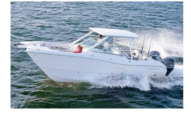
LOA: 27' 6" Beam: 9' 2" Fuel Capacity: 220 gal (2 x 110 gal) Dry Weight w/ Power (Approx): 7,250 lbs (w/ twin 200's) Hull Draft: 14"
