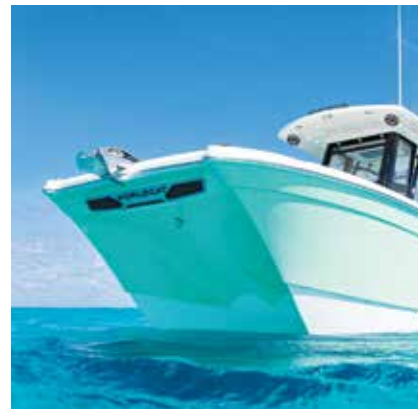
The multihull design of the World Cat 260CC-X delivers a smooth ride in rough conditions and achieves good fuel efficiency and range.
