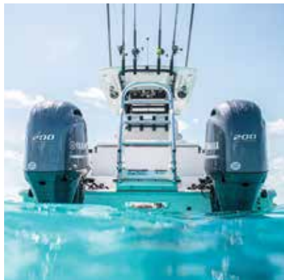
A tilt-up boarding ladder and fixed side rails provide convenient handholds when fishing on the platform that extends between the twin outboards.
