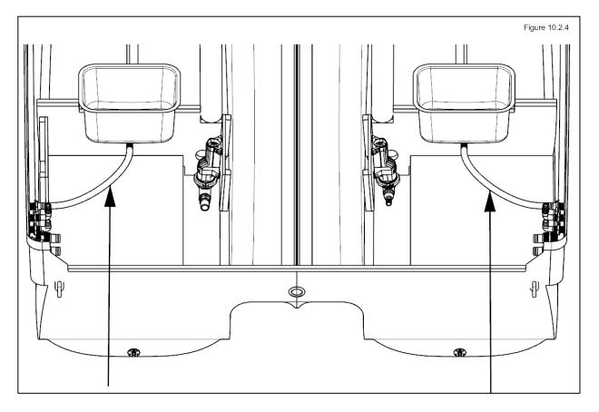
**Fishbox Drains** - The in-floor fishboxes on your World Cat are equipped with dedicated diaphragm pumps to efficiently pump liquids and small solids overboard. The pump and hoses are accessed through the mechanical room lids. (see Figure 10.2.5). The pumps are activated by a switch on the dash (see Figure 10.2.6). See Figure 10.2.7 for hose routing.
