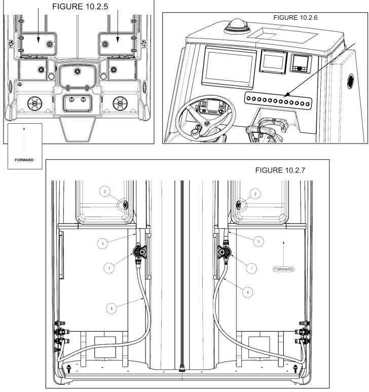
1) Diaphragm Pump 2) Fishbox Drain 3) Hose to Pump 4) Hose Overboard
