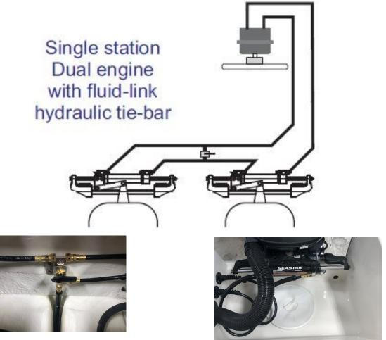
Optional steering system on 235CC, with power steering pump.
