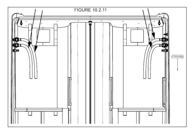
**Livewell System** – The livewell system on your World Cat has been designed to maximize capacity while ensuring proper flow and geometry to keep baits alive longer. Access to the plumbing is gained through the aft deck hatch (see Figure 10.2.12). See Figure 10.2.13 for hose routing.
