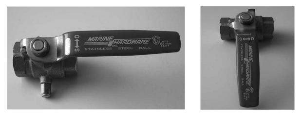
Ball valves (seacocks) are installed on the water intake for both the livewell and raw water system. The seacock must be in the open position for these systems to work. When open, the handle will be parallel to the valve. In the closed position the handle is perpendicular to the valve (see picture above). World Cat recommends that the seacocks remain in the closed position when not in use, or when the boat is left unattended to prevent the vessel from taking on water due to a plumbing failure.
