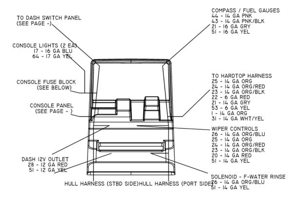
CONNECTIONS TO THE ITEMS SHOWN HERE CAN BE REACHED THROUGH THE ACCESS DOORS LOCATED ON THE CONSOLE BULKHEAD OR BY REMOVING THE ELECTRONICS BOX
